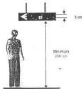
Gambar 2.3.8.2 Standarisasi signage gantung (Sumber: ADA/ANSI Guidelines, Requirements for directional and informational sign, 1999)
